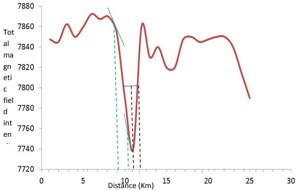
**Fig. 9. Total magnetic field profile along Ikom showing locations of manual depth computed areas**
