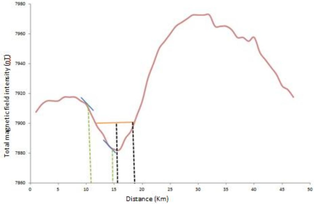
Fig. 11. Total Magnetic Field Profile along Afikpo showing locations of manual depth computed areas
