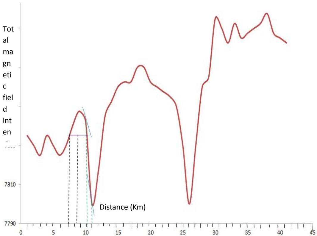
**Fig. 10. Total magnetic field profile along Bansara showing locations of manual depth computed areas**
