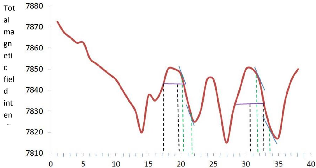
**Fig. 8. Total magnetic field profile along ogoja showing locations of manual depth computed areas**
