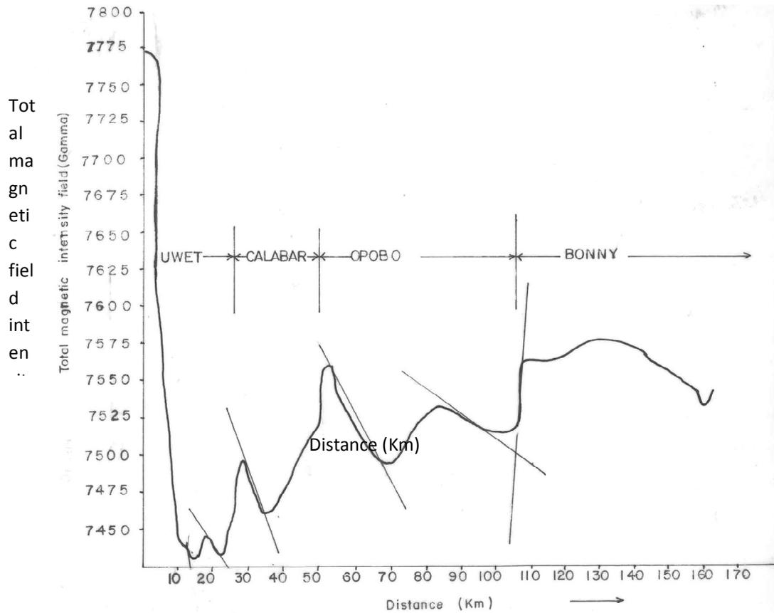
**Fig. 7. Total magnetic field intensity profile from Uwet to Calabar, Opobo and Bonny showing locations of manual depth computed areas**
