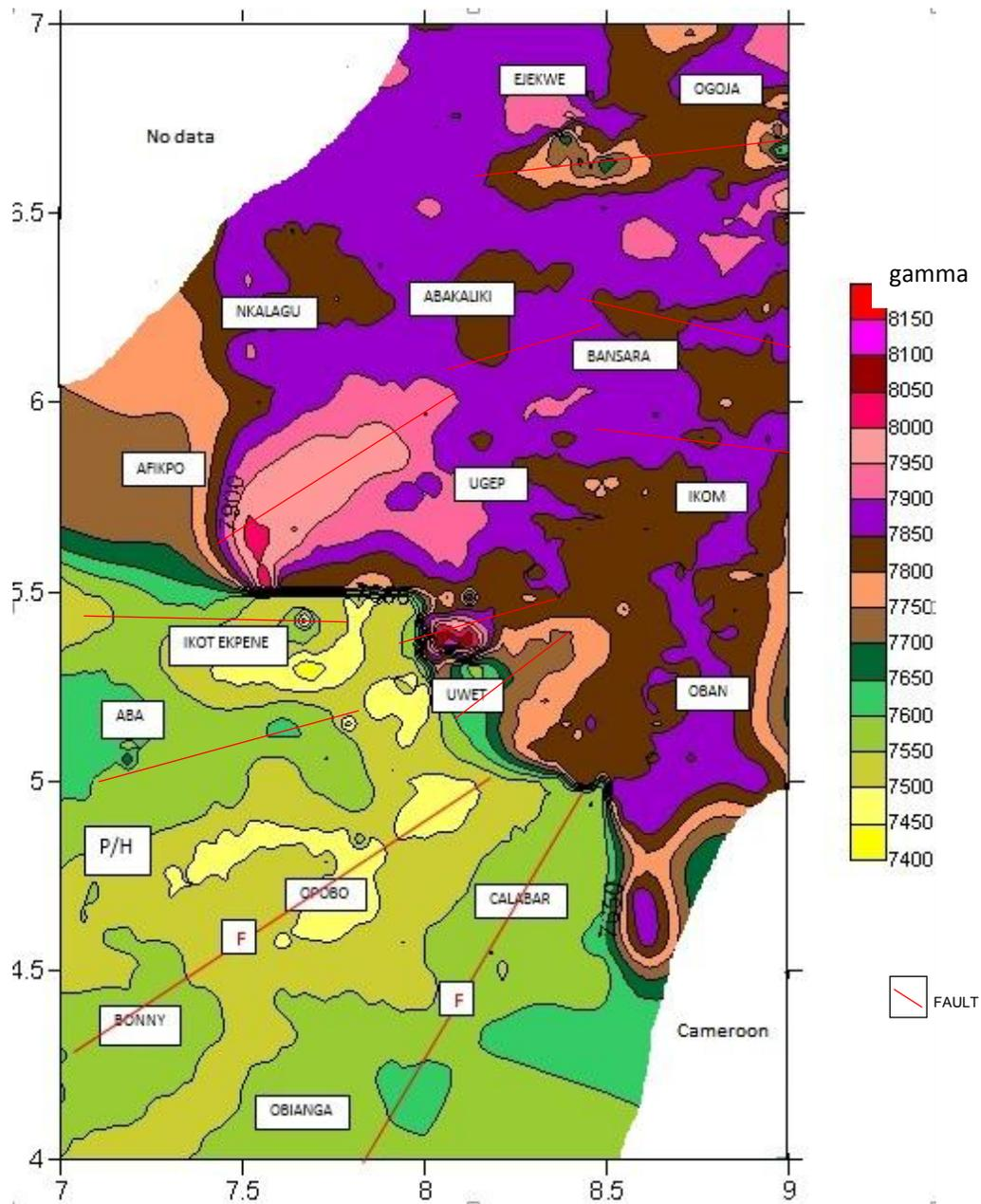
**Fig. 2. Merged coloured total magnetic field intensity map of the study area.( contoured at 50nT )**
