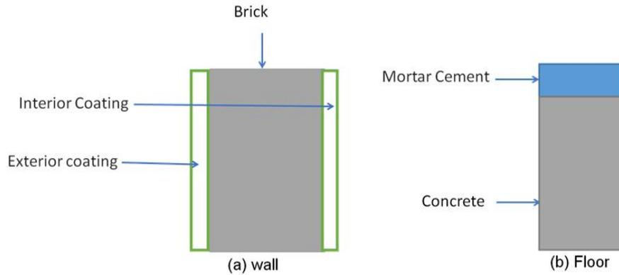
**Fig. 3. Composition of wall and floor**
