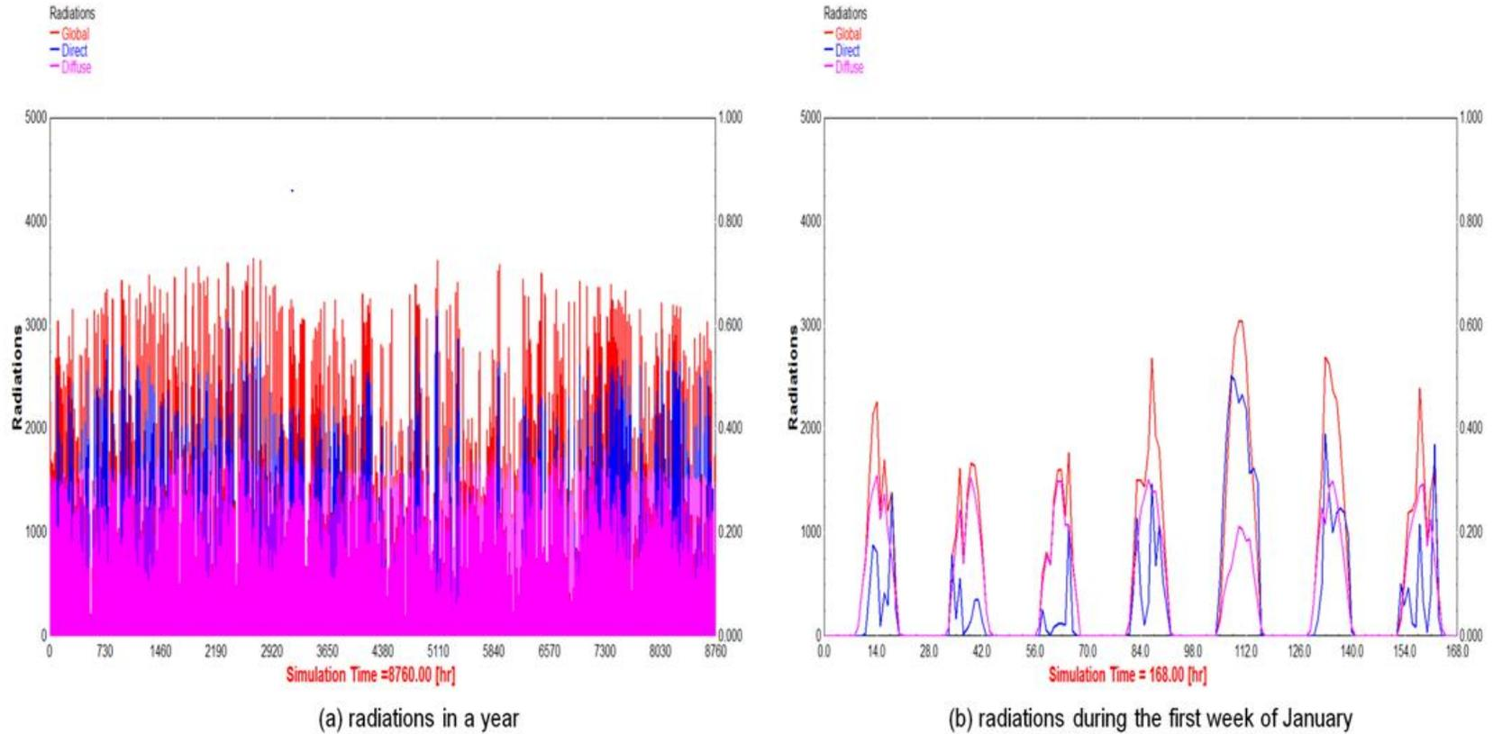
Fig. 6. Global horizontal, diffuse and direct radiation
