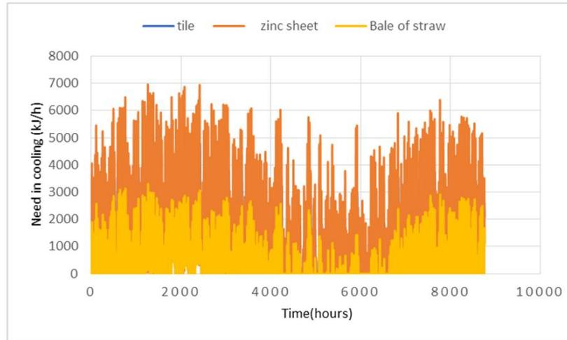
**Fig. 9. Annual need for air conditioning (cooling)**
