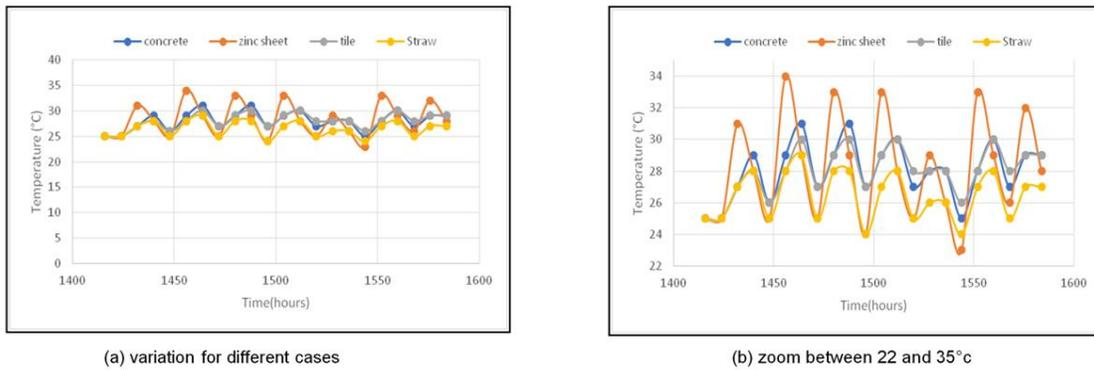
**Fig. 7. Variation of internal temperatures**
