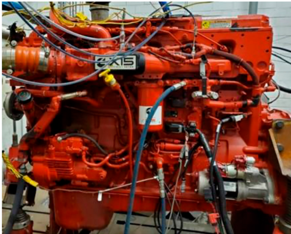
FIGURE 1 Cummins X15 engine platform installed in the test cell.
