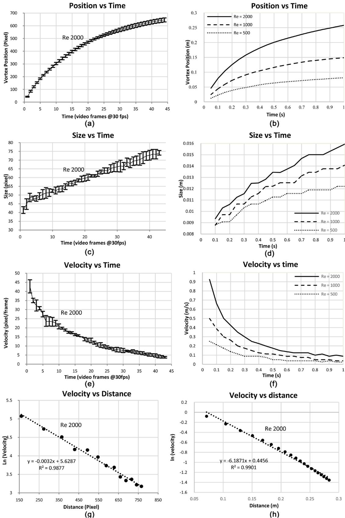
**Figure 4.** Experimental and computational results relating to ring vortex position, size, and velocity. The graphs on the left hand of the page present experimentally measured data. The graphs on the right show directly comparable data obtained by numerical simulation.
