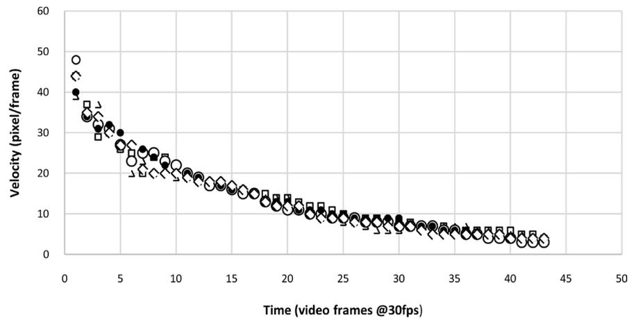
Experimental Results - Vortex Velocity - Reproducibility of 5 vortex rings from the experimental dataset, captured at 30 frames per second (fps)
