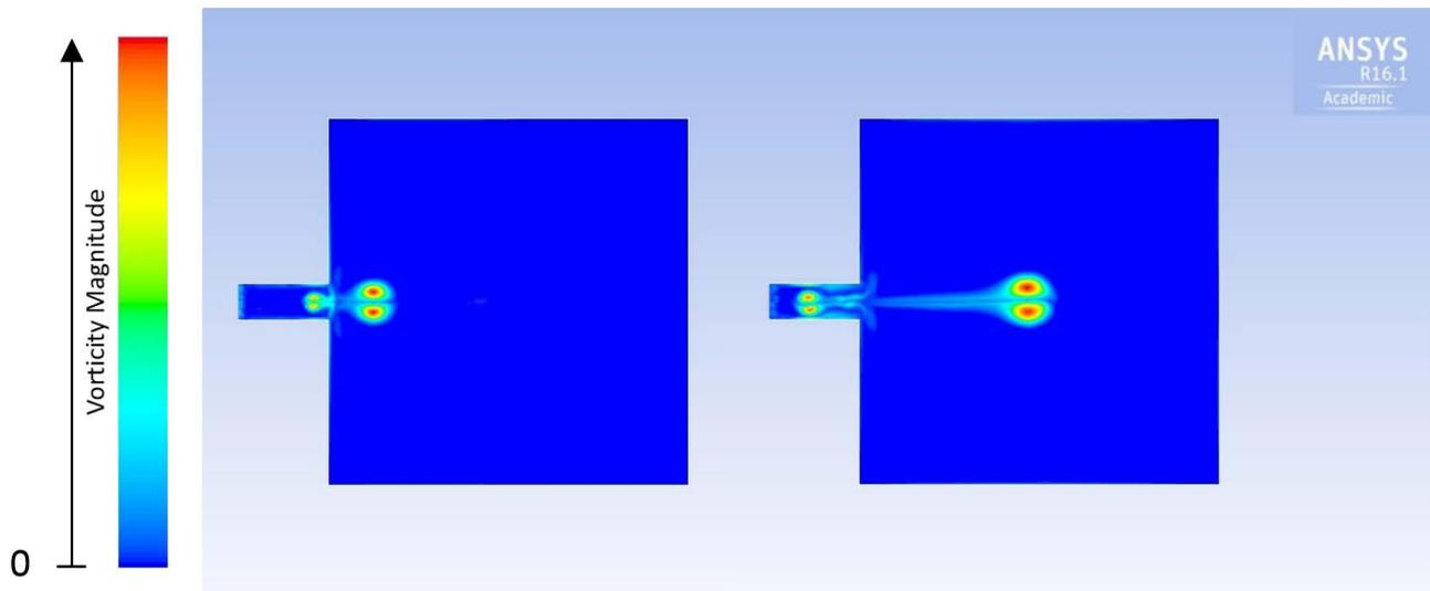
**Figure 3.** Example CFD solutions (2D, axisymmetric) demonstrating generation and propagation of a ring vortex at  $Re = 2000$ . A slug of fluid expelled from the narrow channel at the left of the domain proceeds as a vortex ring that propagates to the right. The images plot vorticity, illustrating complex but stable and predictable flow features.
