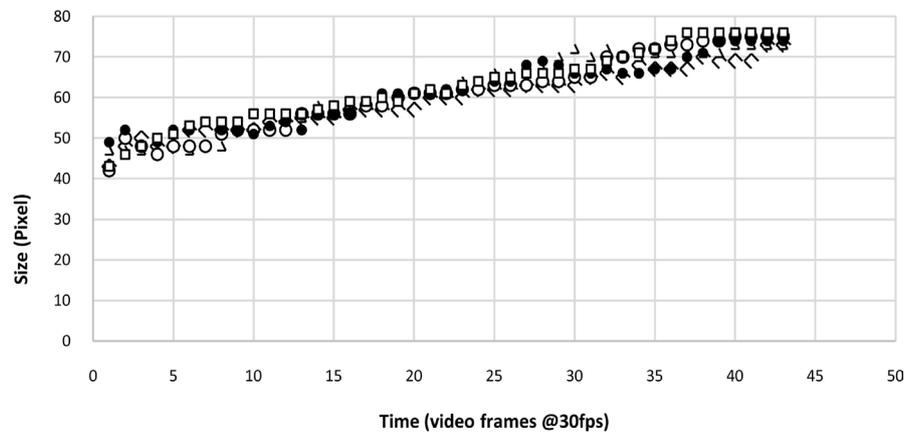
Experimental Results - Vortex Size - Reproducibility of 5 vortex rings from the experimental dataset, captured at 30 frames per second (fps)
