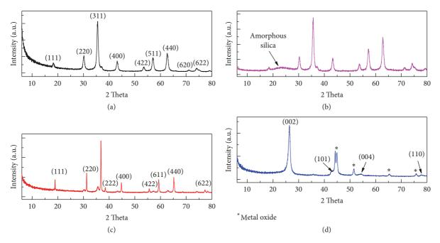
FIGURE 2: XRD pattern of Fe<sub>3</sub>O<sub>4</sub> (a), Fe<sub>3</sub>O<sub>4</sub>@SiO<sub>2</sub> (b), Fe<sub>3</sub>O<sub>4</sub>@SiO<sub>2</sub>-Co (c), and Fe<sub>3</sub>O<sub>4</sub>@SiO<sub>2</sub>-MWCNT (d).
