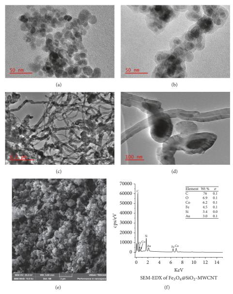
$FIGURE\ 1:\ TEM\ image\ of\ Fe_3O_4@SiO_2-MWCNT\ (c-d),\ SEM\ image\ of\ Fe_3O_4@SiO_2-MWCNT\ (e),\ and\ SEM-EDX\ of\ Fe_3O_4@SiO_2-MWCNT\ (f).$
