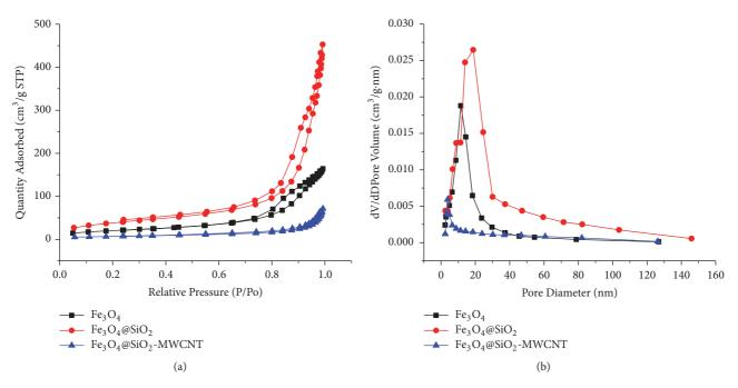
FIGURE 3: Panel (a) is the nitrogen adsorption-desorption isotherm for Fe<sub>3</sub>O<sub>4</sub>@SiO<sub>2</sub>-MWCNT, and panel (b) is the corresponding PSD.
