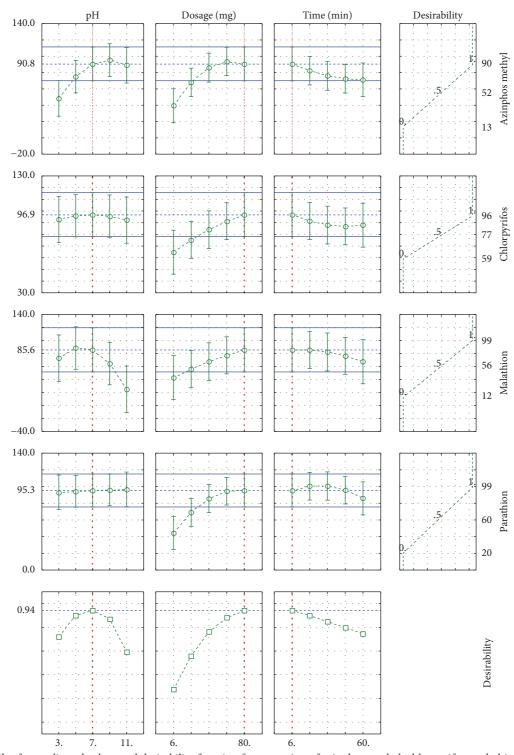
FIGURE 7: Profiles for predicated values and desirability function for extraction of azinphos methyl, chlorpyrifos, malathion, and parathion mix. Dashed line indicated current values after optimization.
