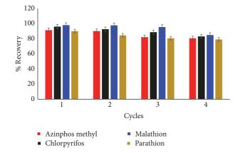
Figure 8: Recycling and reuse of the  ${\rm Fe_3O_4@SiO_2@MWCNT}$  adsorbent in the removal of azinphos methyl, chlorpyrifos, malathion, and parathion mix from aqueous solution.
